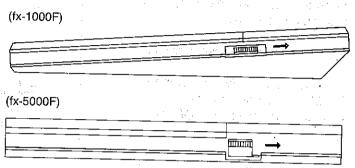
If you turn the dial in the direction shown by the arrow in the illustration, the characters on the display become darker. Turning the dial in the opposite direction makes the characters lighter. If the display is difficult to read even after you make the contrast as dark as possible, it might mean that you need to replace the batteries.
