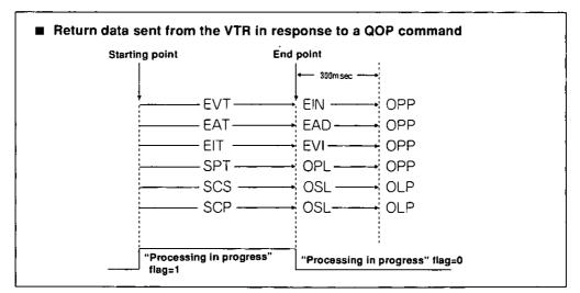
QOS commands are often used to ask the VTR regarding the situation of processing using these commands. For this reason, the timing between the commands and "processing in progress" flag is also shown in the above table.
