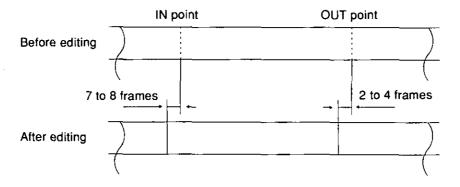
As shown in the above figure, the IN point is -7 to -8 frames and the OUT point is -2 to -4 frames. (The above figure shows the difference between the edit points.)
