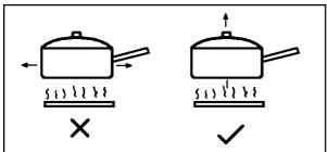
Avoid placing fish kettles or large preserving pans across two hotplates as this may cause damage.
