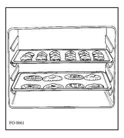
The oven has four shelf levels, and is supplied with two anti-tip shelves.
