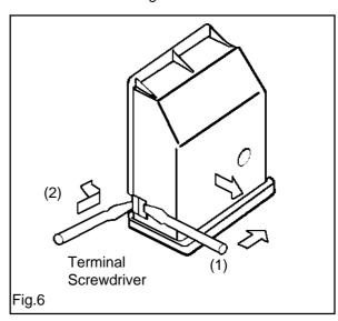
Lift cover and remove screw from cable clamp.
