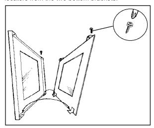
5. Clean the outer and inner glass using hot soapy water or Hob Brite. DO NOT try to clean the aluminium foil which is inside the door. The foil is there to help keep the door cool, if it is damaged it will not work. Ensure that all parts are well rinsed and thoroughly dry before attempting to replace the outer door glass.
