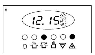
Note: When the automatic timed period starts, the oven neon will cycle ON and OFF during cooking.
