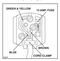
Connect the Green and Yellow (earth) wire to the terminal in the plug which is marked with the letter  $^{\text{K-}}$  or the earth symbol  $\oplus$  or coloured green and yellow.
