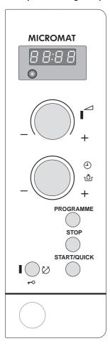
1. Press the START-button 'START/QUICK' three times. The time appears in the display and the programme begins. The microwave power signal lamp comes on.
