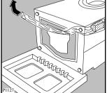
5. Set the machine upright and remove the remaining rear screw. Slide out the relevant pin.
