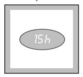
The delay time is displayed for 3 seconds, then the duration of the selected programme reappears. After you have pressed the START/PAUSE button, the countdown begins, and the delay time value decreases by one unit every hour.
