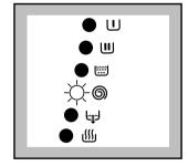
To select **Drain** press the SKIP button three times, the **wash - rinse - spin** LED,s go out.
