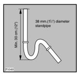
When discharging into a standpipe ensure that the top of the curve in the hose end is no more than 90cm (35.4") and no less than 60cm (23.6") above floor level. The upright standpipe should have a minimum length of 30cm (12") from the bottom of the elbow to the top of the pipe (see diagram).
