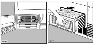
It is quite normal to find droplets of water on top of or at the front of the condenser unit. This is not a fault with the appliance. Clean it with a brush and rinse it under the shower if necessary.
