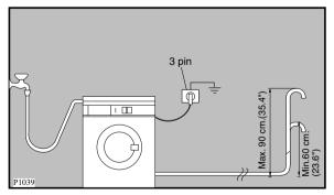
Make sure that it is designed in such a way, that the end of the drain hose cannot be covered with water. The drain hose may be extended to a maximum of 4 metres. An additional drain hose and joining piece is available from your local Service Force Centre. The joining piece must have an internal diameter of 18mm. If you intend the drain hose to empty into a sink, make sure that the sink is empty and the plug hole is not blocked. Use the plastic "U-Piece" supplied.
