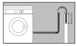
The standpipe should have an internal diameter of approximately 38mm (see diagram) thus ensuring there is an air break between the drain hose and standpipe.
