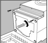
Set the machine upright and remove the two remaining bolts from the back.
