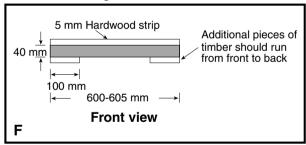
Drill four fixing holes (see Fig. G)
