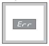
• An alarm code indicates a fault in the machine operation (see the relevant chapter on page 21-22).
