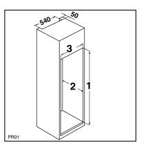
Fit the appliance in the niche by making sure that it stands against the interior surface of the unit on the side where the door hinges of the appliances are fitted. Insert the appliance until the upper strip butts up against the unit (1) and make sure that the lower hinge is in line with the surface of the unit (2).
