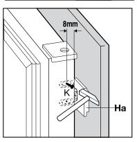
Place the small square on the guide again and fix it with the screws supplied.
