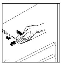
Unscrew the light cover and then pull it outward by pressing as shown in the figure. Unscrew the bulb and replace it with one of the same power (the maximum power is shown on the light diffuser) available from your nearest Service Force Centre.
