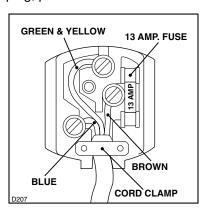
Connect the Green and Yellow (earth) wire to the terminal in the plug which is marked with the letter
