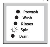
To select **Drain** only, press the "**Skip**" button three times, the **wash - rinses - spin** LED,s go out. The **Drain** LED only remains alight.
